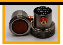
Features: Delayed contact ultrasonic transducer with polystyrene replaceable delay tip. Constructed with stainless steel housing and side mount BNC connector on "G" Series and side mount microdot (10-32) connector on the "W" and "K" series.
