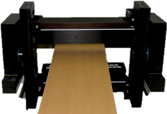
32 channel brick array setup for online inspection
