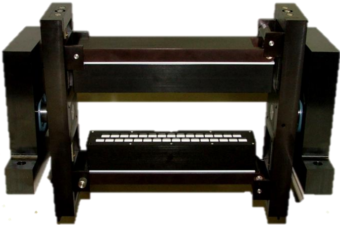
32 channel brick array setup for online inspection
