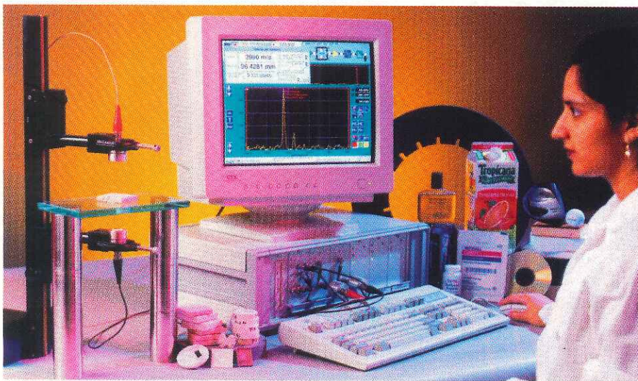
Figure 1. Ultrasonic non-contact analysis system, shown here with non contact transducers and a green ceramic tile sample (left).
