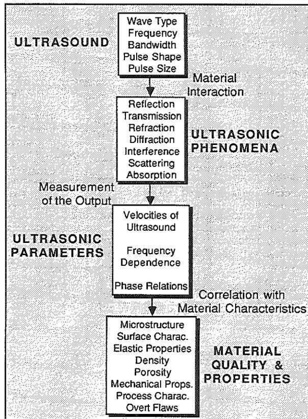
Figure 1 - Principles of ultrasonic NonDestructive Characterization (NDC) - applications of ultrasound-material interaction phenomena for materials quality and properties analysis.
