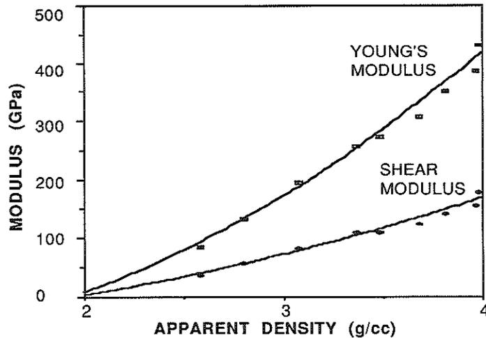
Figure 5 - Young's and shear moduli of elasticity as functions of density of sintered alumina generated from ultrasonic velocities data.
