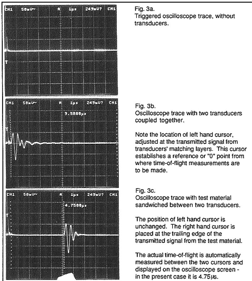
Figure 3 - A sequence for accurate time-of-flight measurement by direct transmission dry coupling mechanism.
