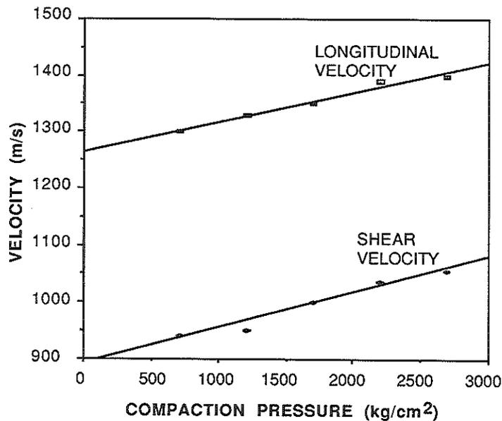
Figure 7 - Relationship between compaction pressure of green alumina and its longitudinal and shear wave velocities established by direct transmission dry coupling methods
