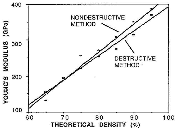
Figure 6 - Comparison of destructively (4-point bending method) and ultrasonically determined Young's modulus of alumina as functions of its density.
