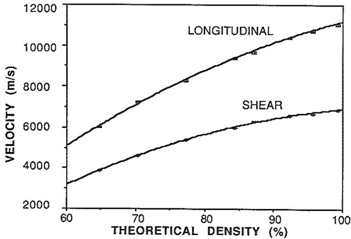
Figure 4 - Relationships between the density and longitudinal and shear wave velocities of sintered alumina determined by direct transmission dry coupling methods. Frequency of longitudinal wave transducers: 10MHz. Frequency of shear wave transducers: 5MHz.
