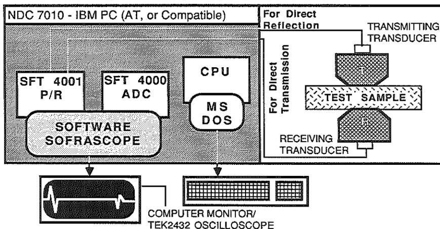
Figure 2 - Pulsed ultrasound setup of NDC 7010 used for the measurement of longitudinal and shear velocities by dry coupling methods.
