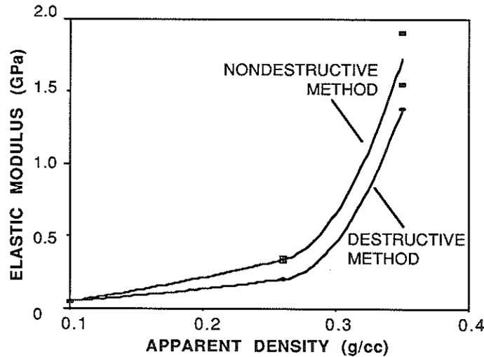
Figure 8 - Comparison of destructively and nondestructively determined elastic moduli of "ultra" porous rigid ceramics in thickness direction as functions of density.
