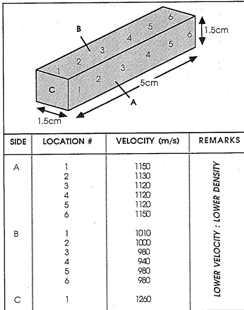
Fig. 15. Velocity variations at different points - presumably indicative of density or binder content variations in a green ferrite component (composition, unknown). Here, each test point corresponds to 6mm diameter.
