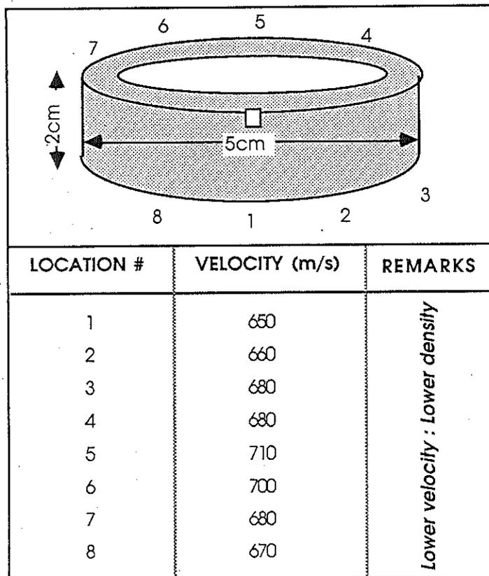
Fig. 16. Velocity variations at different points - presumably indicative of density or binder content variations in another green ferrite component (composition, unknown). Each point of test here corresponds to 3mm diameter.
