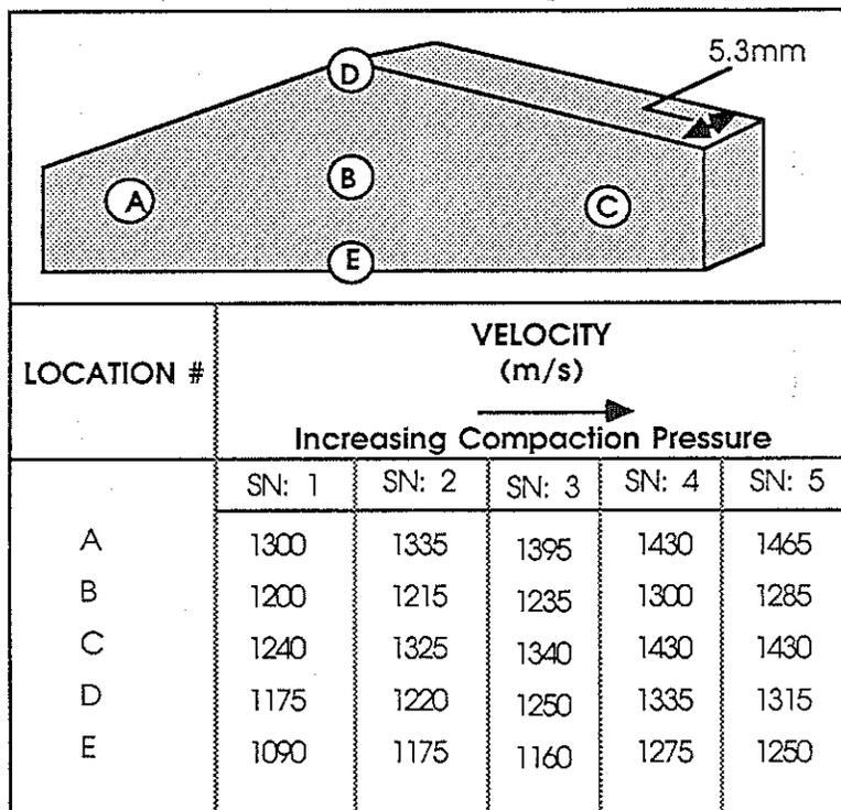
*Fig. 17. Velocity variations at different points in a green WC component as a function of compaction pressure - at ~ 0.25 ton increments between various samples. Each point of measurement in this case corresponds to 6mm diameter.*
