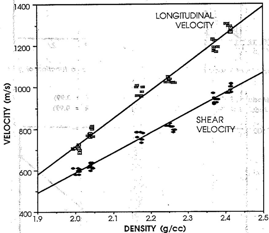
Fig. 8. Relationship of longitudinal and shear wave velocities with green  $Al_3O_3$  density.
