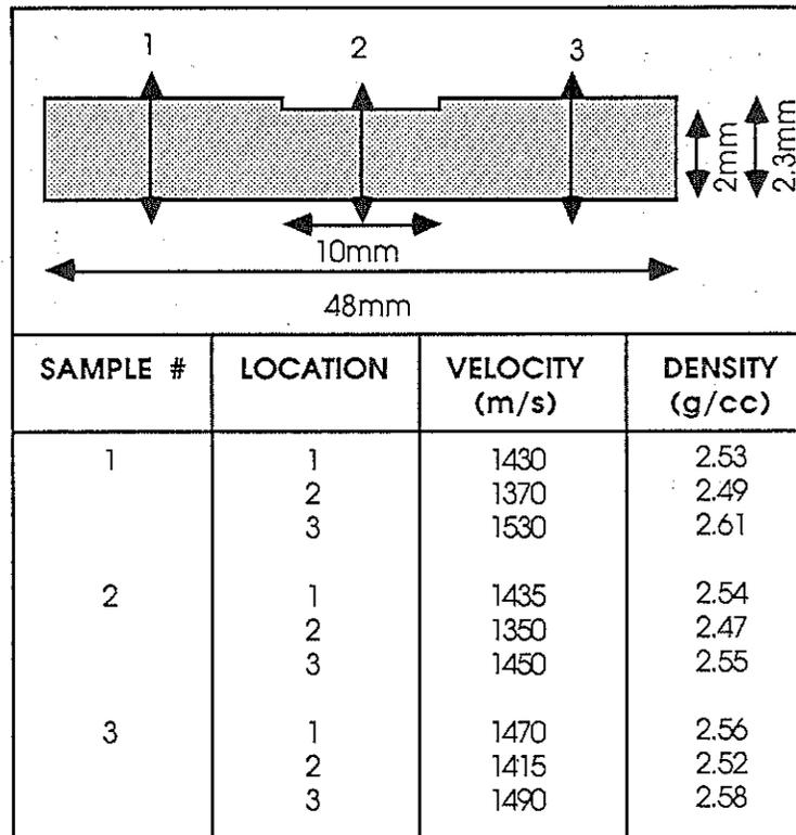
Fig. 13. Ultrasonically determined density (from relation in Fig. 9) of green alumina substrates at various locations. Here, each point of measurement corresponds to 6mm diameter.
