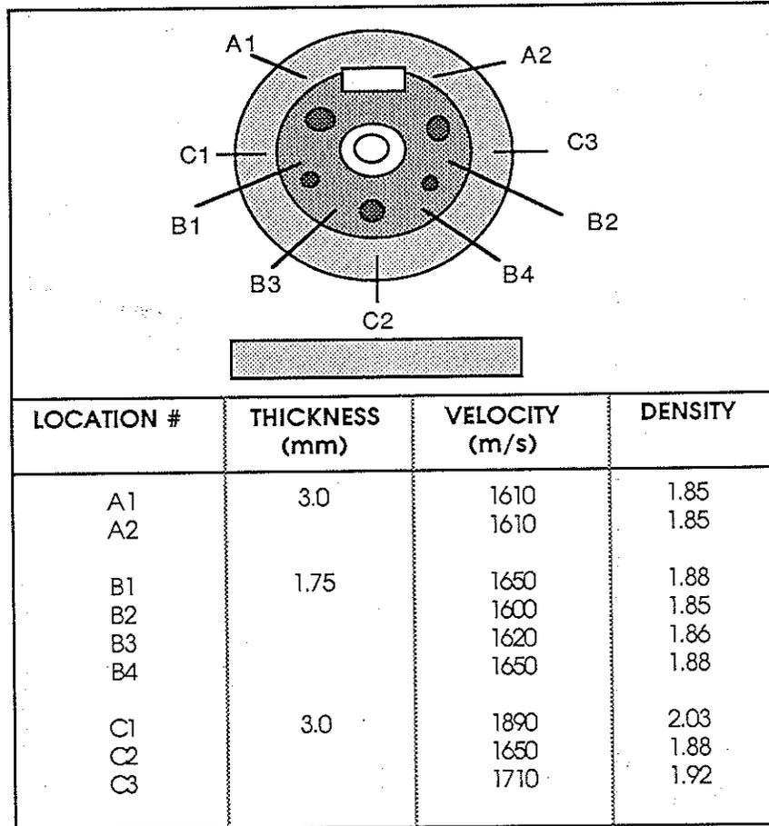
Fig. 14. Ultrasonically determined density (from relation in Fig. 11) of green steatite component at various location. Point of each measurement here corresponds to 3mm diameter.
