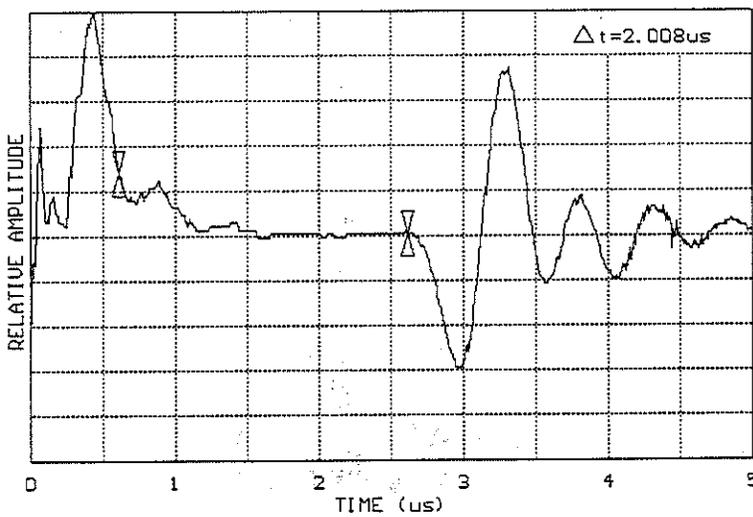
Fig. 7. Propagation of shear ultrasound through green  $Al_2O_3$  (2.4mm).
