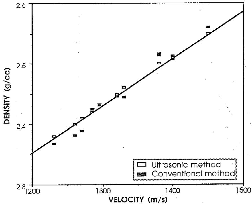
Fig. 12. Comparison of ultrasonically determined and measured density of green  $\text{Al}_2\text{O}_3$ .
