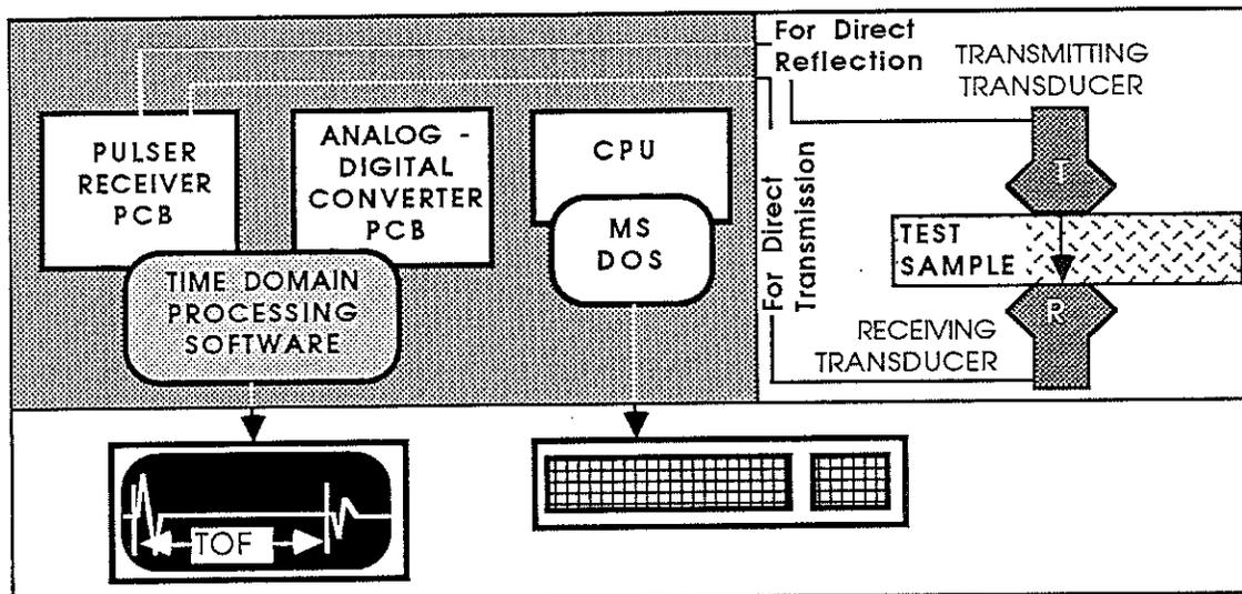
Fig. 2. A schematic layout of pulsed ultrasonic set up and transducers configuration used for nondestructive characterization of green materials.
