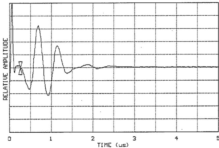
Fig. 4. RF trace with transmit and receive transducers touching each other. Note the position of left hand cursor, indicating "zero" reference point.
