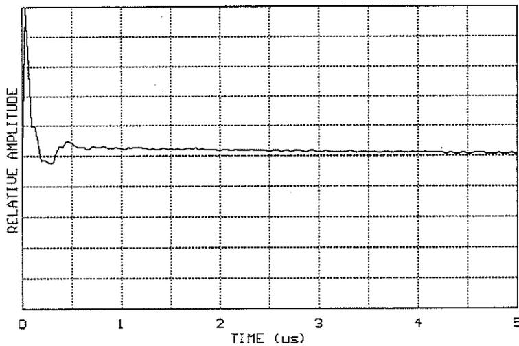
Fig. 3. RF trace without transducers.
