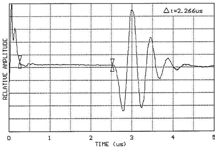
Fig. 5. RF trace with example material (6mm) sandwiched between the transducers. Note the position of right hand cursor, indicating the transmitted signal through material.
