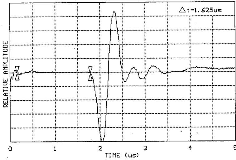
Fig. 6. Propagation of longitudinal ultrasound through green  $Al_2O_3$  (2.4mm).
