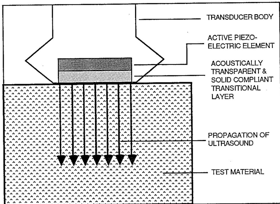
Fig. 1. A schematic cross-section of a dry coupling ultrasonic transducer showing the propagation of ultrasound into a test material.
