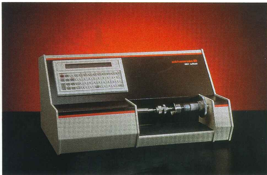
Micromeritics' Geo-Pyc was used for the compacted powder measurements.
