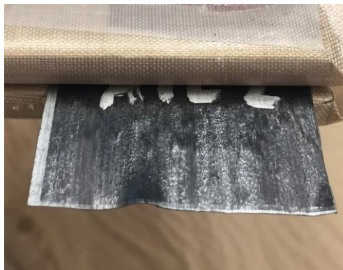
Figure 4. Prepreg Specimen between Teflon-covered Clamped Plates for Water Pickup Test
