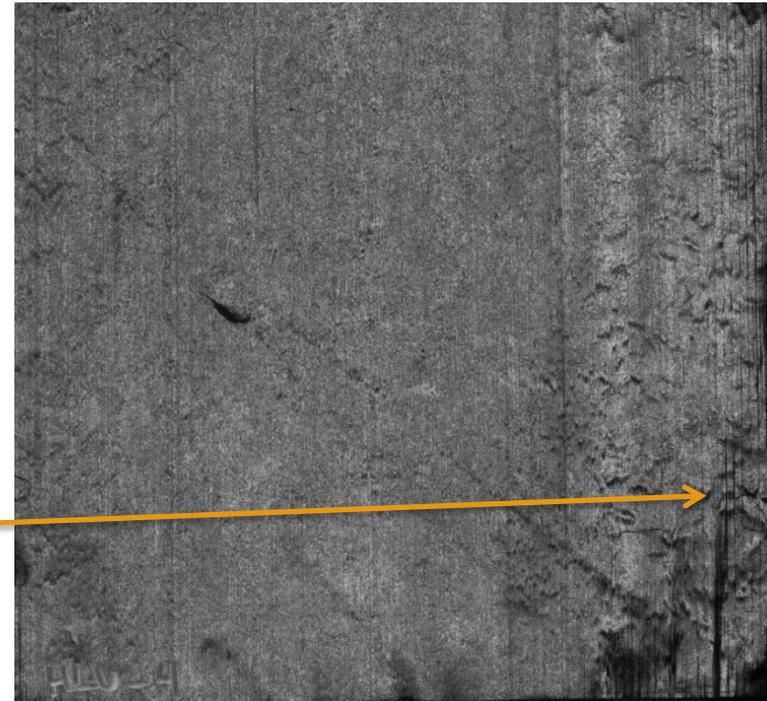
Section on right side of sample appears optically shiny, while transmittance is especially low. This may be due to resin which is not properly impregnated in this region, and remains upon the sample surface
