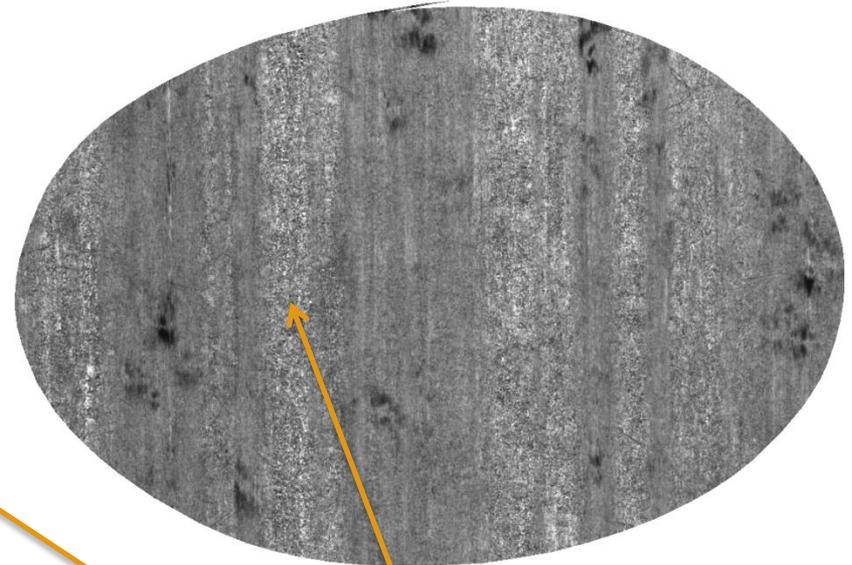
Low transmittance stripes appear “shiny” in optical image. May be due to resin which was not impregnated into fiber bed (still remaining on prepreg surface)
