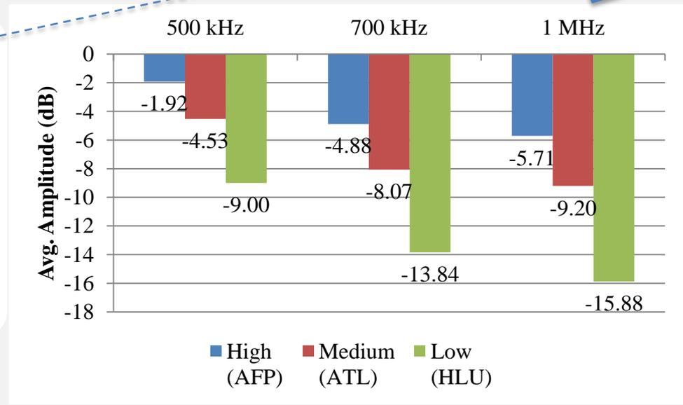
Lower frequencies exhibited some saturation in measurement and lower sensitivity to change in LOI. 2 MHz exhibited some areas of no signal amplitude
