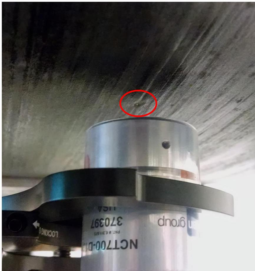
The presence of pin-holes allows for abnormally high ultrasonic transmission, which must be filtered out in real-time or post-processing
