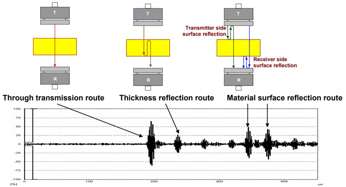
Fig. 2. Mode of ultrasound propagation in direct transmission. Shown here are various routes in this mode and their significance with respect to material.
