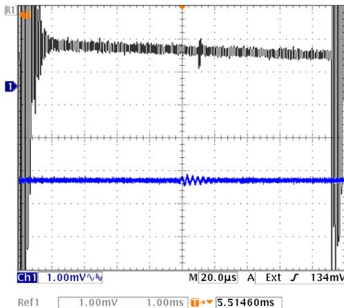
Fig. 7. Reflection from a flat surface located at 1 m From 500 kHz, 19x19 mm transducer. Excitation: -200 V spike. Amplification: NONE.
