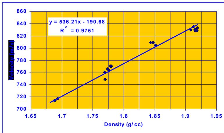
Fig. 3. Velocity-density relationship for green alumina
