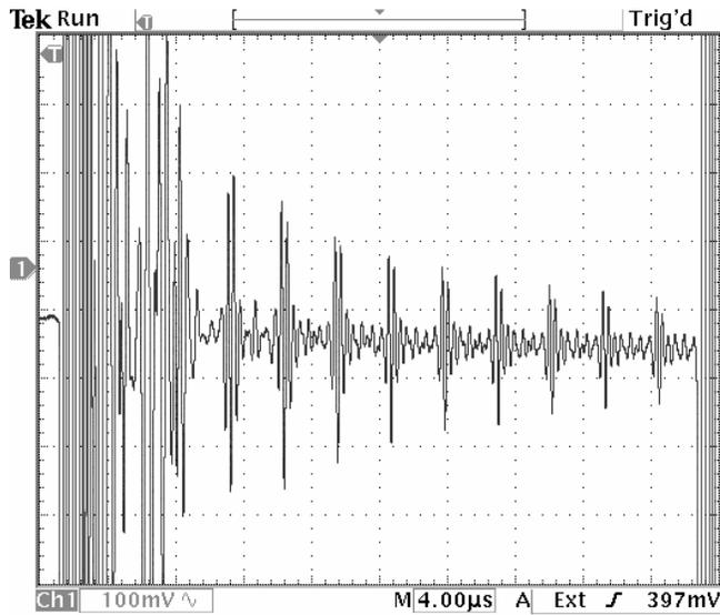
Fig. 10. Pulse-echo multiple reflection from a 10 mm steel block at 50 bar air pressure. By permission
