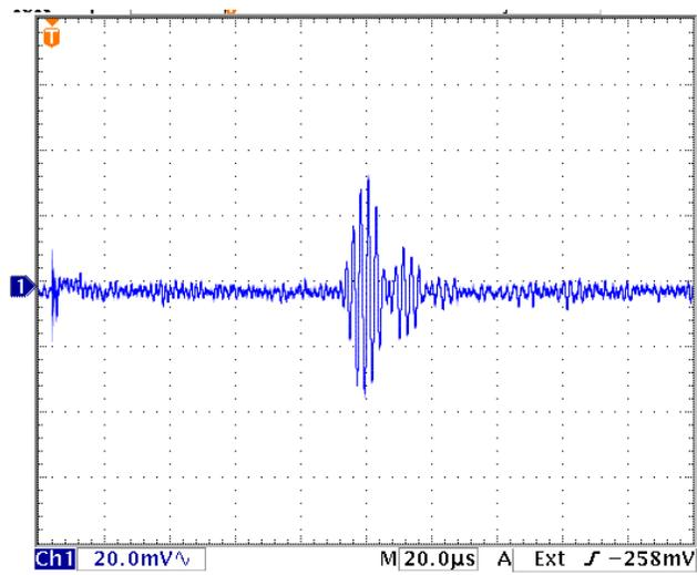
Fig. 12. Surface wave in steel
