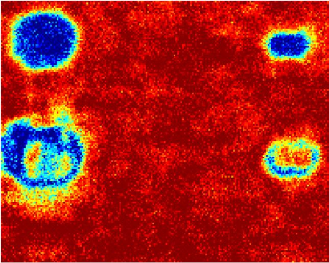
.Fig. 13. Same side image from a 2mm CFRP-NOMEX interface with embedded defects.
