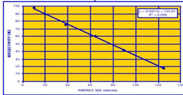
Fig. 8. Reflectivity as a function of particle size
