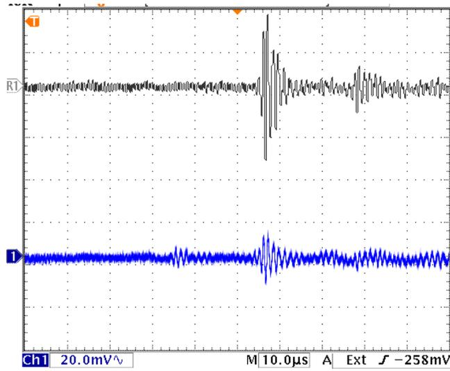
Fig. 11. Same side defect-free (top) and defective (bottom) 3.0 mm cylindrical hole) regions in a 50 mm polystyrene block
