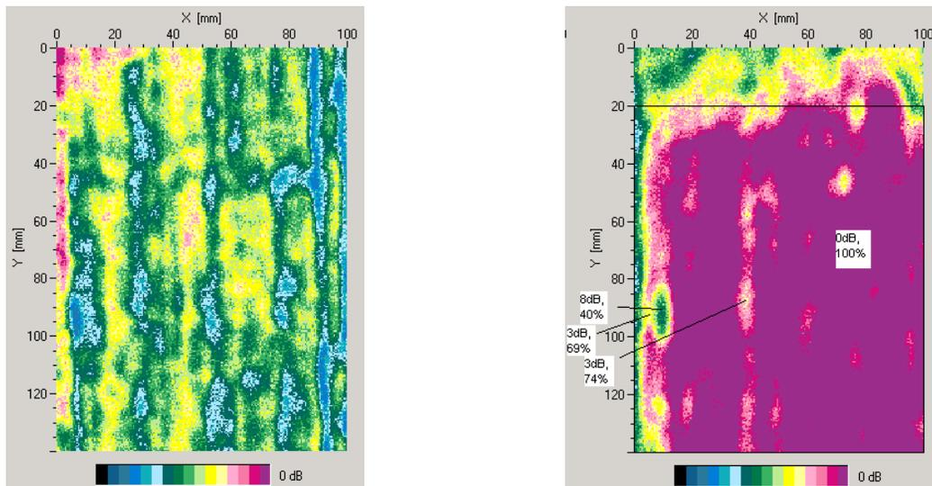
Fig. 5. 500 kHz NCU images of uncured consolidated (left) and cured CFRP composite. Lighter regions in the cured material indicate porosity, also detected before curing. By permission from HEXCEL Composites, UK.
