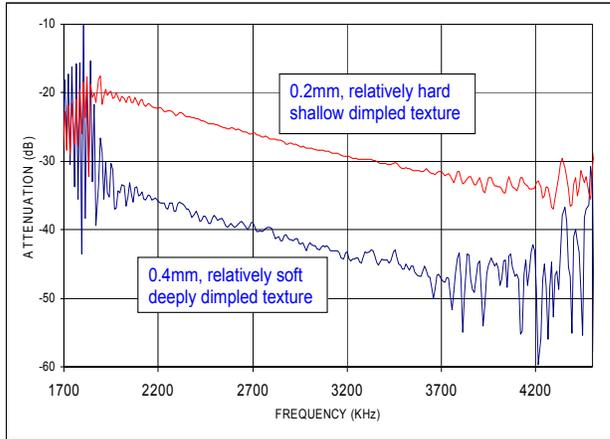
Fig. 6. High frequency NCU spectroscopy of paper for texture analysis
