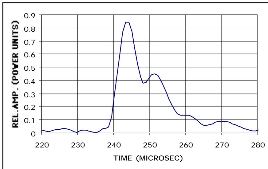
Fig. 13. NCA-1000 With 1MHz Non-Contact Transducers. Transmission signal through 3mm Rocket Motor Insulation Bonded to 12mm Steel.
