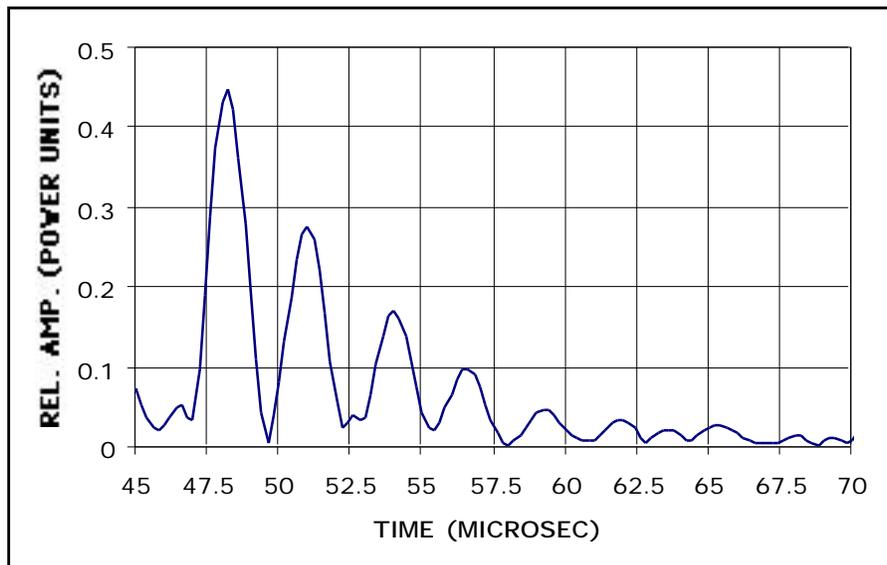
Fig. 7. Transmitted signal through 4.7mm thick multi-layer graphite fiber plastic composite generated by non-contact technique in ambient air @ 2MHz with NCA-1000. First peak is directly transmitted through the material. Rest of the peaks correspond to reflections from two sides of the material. Compare with Fig. 6.
