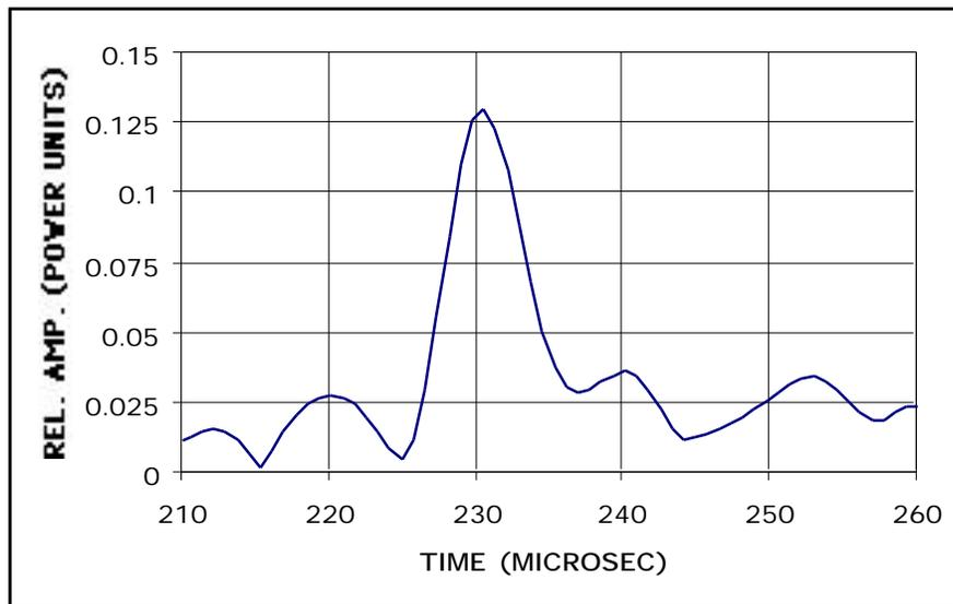
**Fig. 11. NCA-1000 With 1MHz Non-Contact Transducers. Transmission signal through 25mm Composite-Laminated Kevlar Honey-Comb Composite.**
