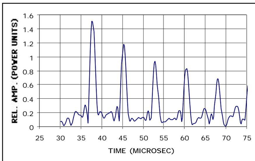
Fig. 5. Transmitted signal through 9mm thick polystyrene generated by non-contact technique in ambient air @ 2MHz with NCA-1000. First peak is directly transmitted through the material. Rest of the peaks correspond to reflections from two sides of the material. Compare with Fig. 4.
