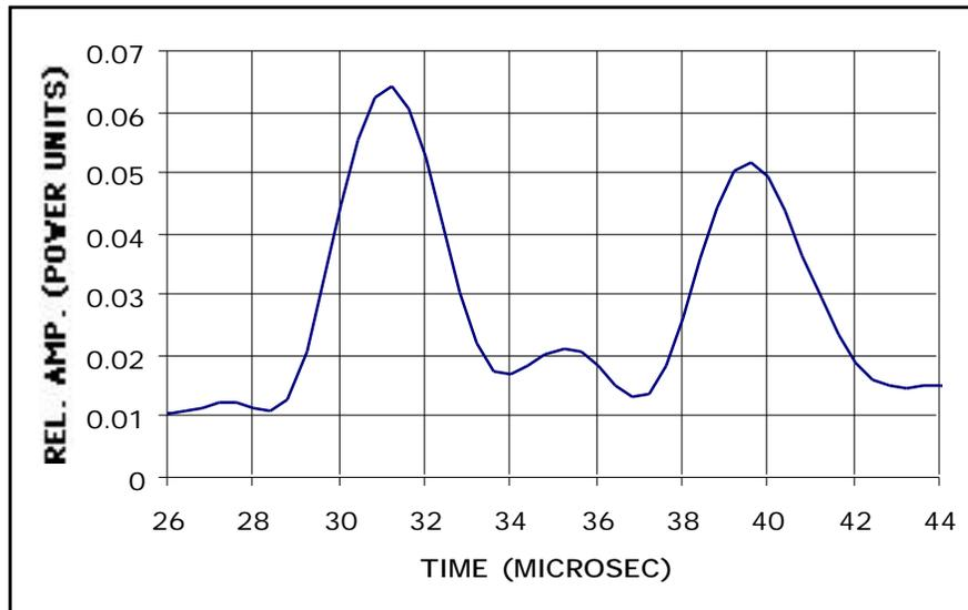
Fig. 9. NCA-1000 With 2MHz Non-Contact Transducers. Transmission signal through 25mm Carbon Steel. First peak, directly transmitted through the material, the next one corresponds to reflection through its thickness.
