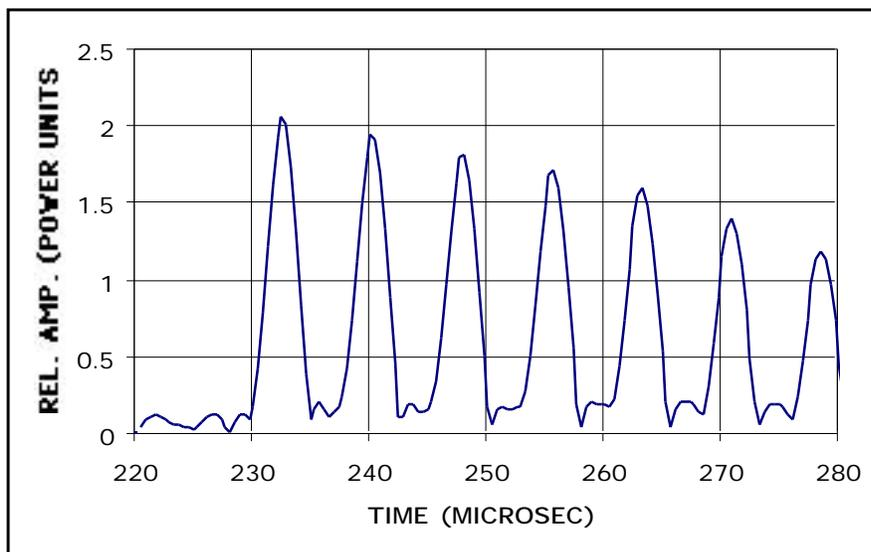
Fig. 15. NCA-1000 With 1MHz Non-Contact Transducers. Transmission signal through 9mm Polystyrene Sheet.
