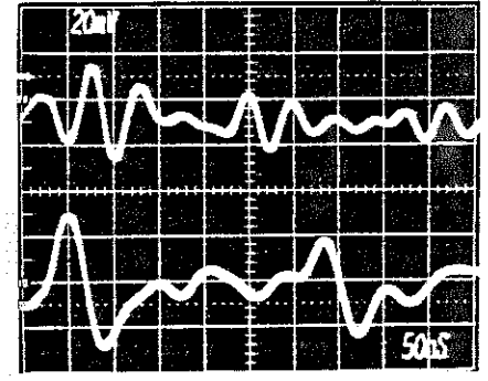
Fig. 6. Real time oscilloscope traces of longitudinal ( top ) and shear ( bottom ) waves from dense \text{BeO} (porosity: none, grain size: sub-micrometer, thickness of the material investigated: 1.07 mm; longitudinal transducer: 6 mm diameter and 20.0 MHz, velocity: 12 190 m/s; shear wave transducer: 6 mm diameter and 10.0 MHz, velocity: 7360 m/s, elastic modulus: 396 GPa, shear modulus: 162 GPa, and Poisson's ratio: 0.21).
