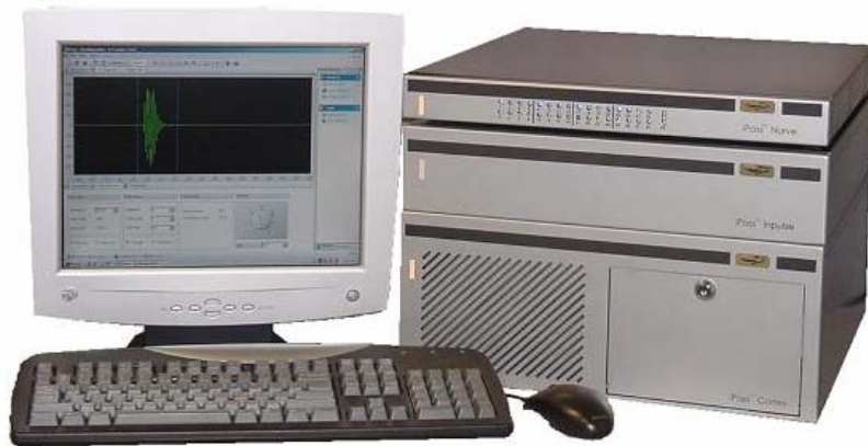
Fig. 1 The iPass Non-Contact Ultrasound system composed of variable frequency and pulse-width pulser, multi-channel receiver, and CPU for the evaluation of temperature and moisture content of lumber.
